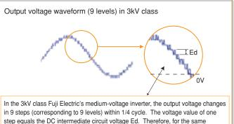
voltage output, a larger number of steps means a smaller voltage value at one step. Thus, Fuji Electric's inverter can also reduce the surge voltage appearing at the motor terminal and thereby moderate the stress applied to the motor.
