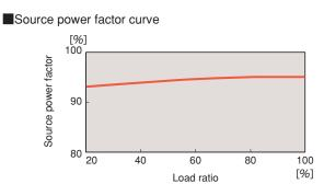
Note: The efficiency and power factor data on this page are calculated by assuming that a 315kW motor is operated at the rated speed with a 3.3kV-input, 390kVA-output inverter. The data on efficiency is obtained using Fuji Electric's standard 4-pole motor
