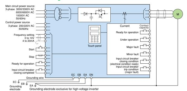
Note: Be sure to use an EA grounding electrode exclusive for the high-voltage inverter, and isolate it from the main grounding lines of other devices.
