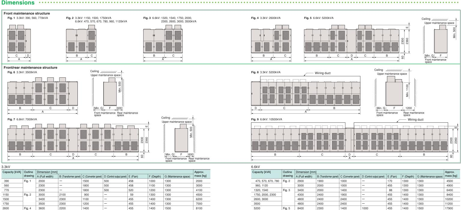
Notes: (\*1) The outline dimensions of the panel represent the maximum dimensions of a standard-capacity model.
